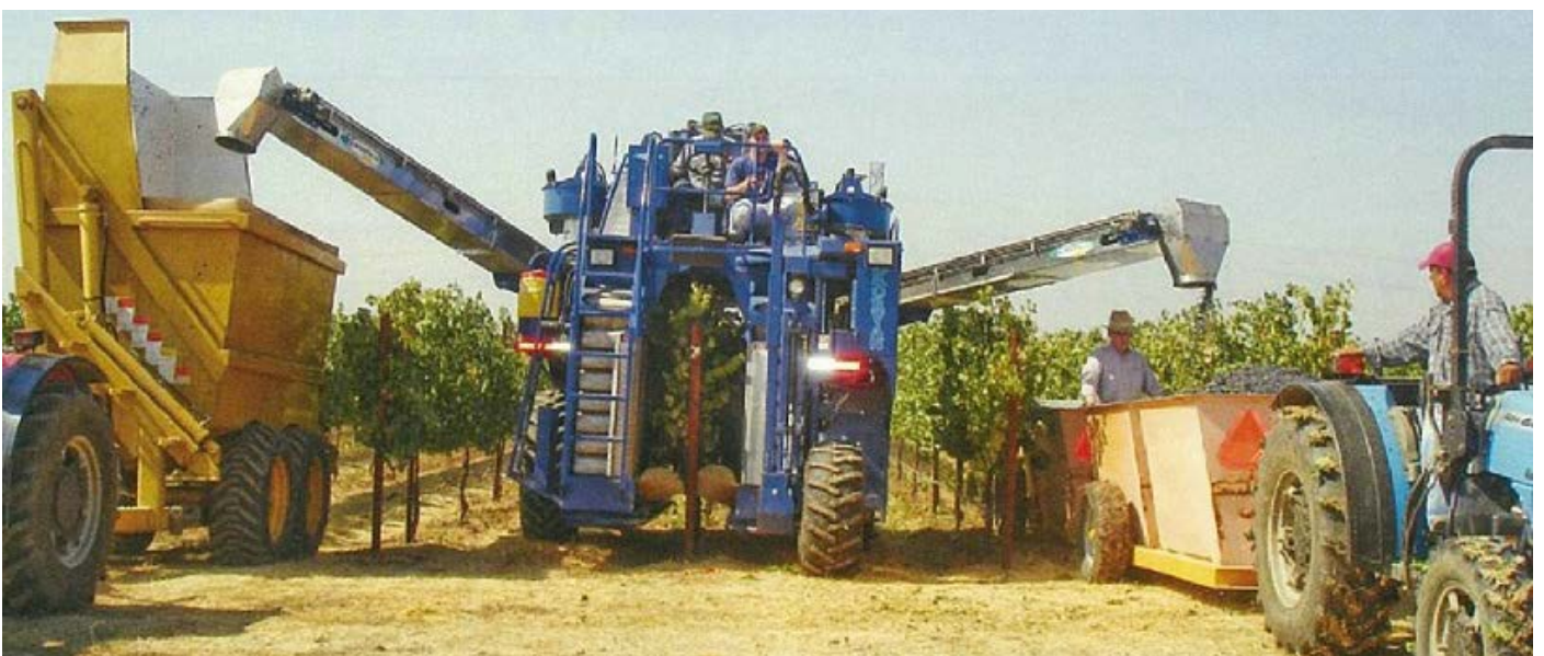
Figure 1: Adapted harvester with two gutters to deposit grapes from different zones with different grape quality grades, as identified by NDVI images into the pressing bins. (Kurtural et al. , 2011)
