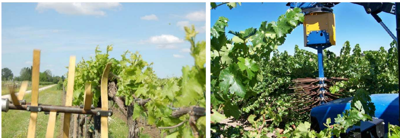
Figure 2: Example of a machine which thins summer shoots on cordon systems (left) and a machine which applies crop control by shaking clusters off (right). (Intrieri, 2013; Dokoozlian, 2013)
