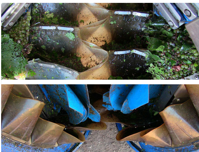
Figure 3: Mechanical harvester which works with collection bowls (top). These collection bowls also serve as double conveyers (bottom) that carry the grapes to the load bin on the machine. (Photo: Robert Stolk)
