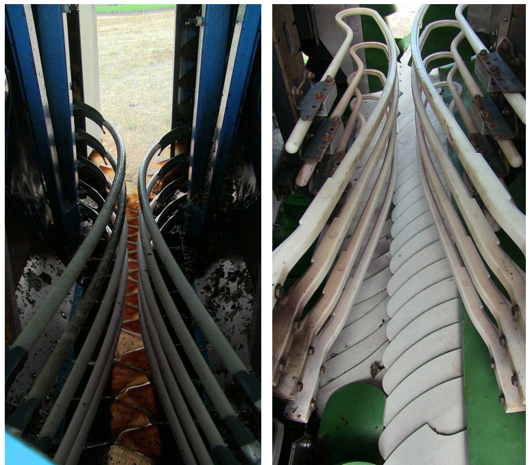
Figure 1: The harvesting chambers of different mechanical harvesters which use a horizontal shaking mode and bow rods. (Photo: Robert Stolk)
