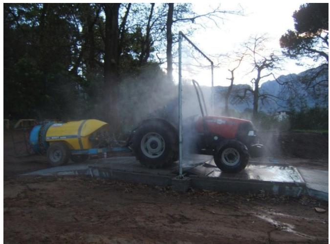
Figure 5: Clean implements with high pressure water and mild detergents before entering healthy vineyards, especially if implements have been in leafroll infected vineyards prior to that. (Image: G. Pietersen, ARC-PPRI)
